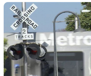
The all familiar “crossbuck” will be a staple at all our street level crossings. This universal sign is used the same as a yield sign and motorists must yield at the grade crossing if a train is approaching.
