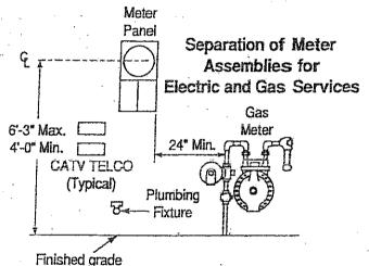
Plumbing fixtures which extend more than 6" out from wall surface must be located 18" minimum from the outside edge of the meter panel.
